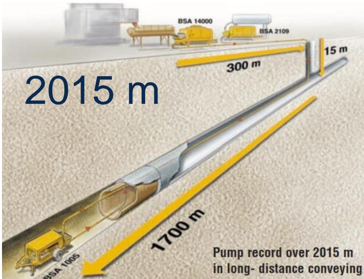
Pump record over 2015 m in long-distance conveying
